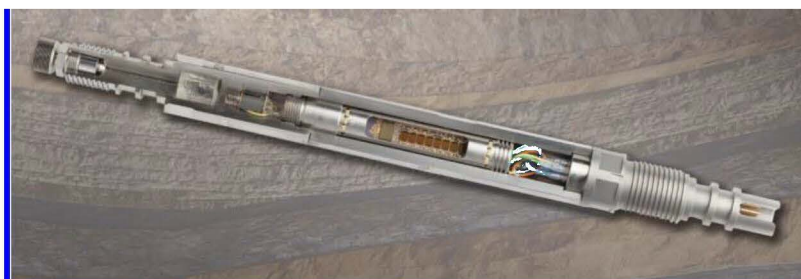
Figur 30 – Gauge used for production (SLBs Signature-måler)
